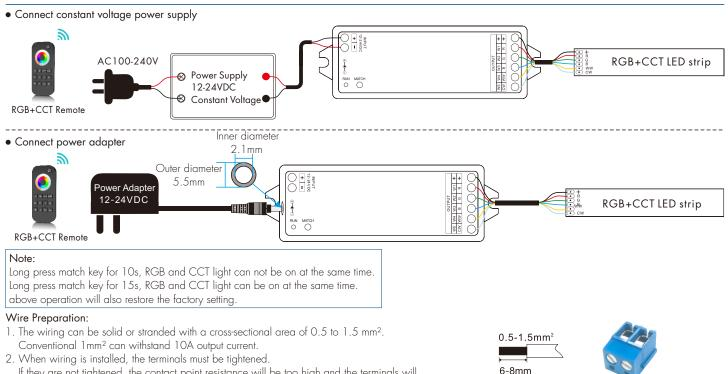
If they are not tightened, the contact point resistance will be too high and the terminals will easily burn due to heat when used at full load for a long time.
